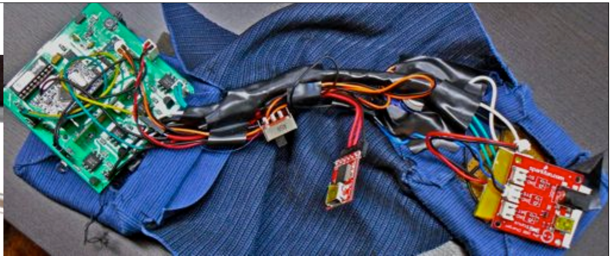
'Internals' of folding display control boards, sensors, and muscle wire activation.
