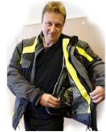
CyberJacket: A heavy duty Hein Gericke jacket for use in the field. Equipped with a CardPC, dGPS and GSM 'phone. User interface is audio (speech recognition & TTS) and/or a Jornada hand held display.
